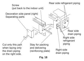
After piping is finished, cut the removed penetration cover along the shape of piping, and install.
